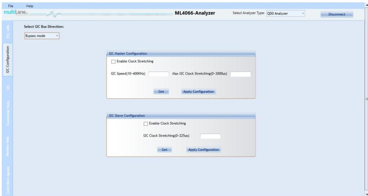
When choosing **Internal Slave**, the user can Read/Write the Data of the Analyzer’s EEPROM. **Internal Master** allows User to read/write on the Module.
