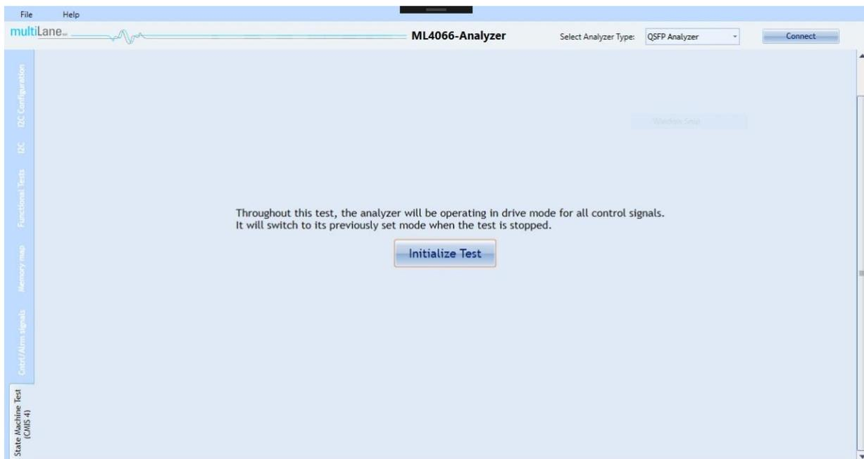
Upon test initialization, the CMIS compliance version is verified and module type is detected. If the latter was not feasible the test would not start normally.
